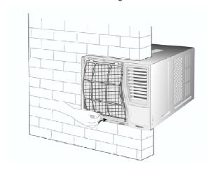
• Slide the front intake grille slightly to the right to reattach the tabs and then push it down to close tight
